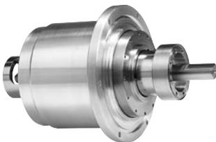
Ferrotec offers multi-axial feedthroughs for wafer handling applications. These offer extremely high repeatability with zero backlash. Linear motion can be incorporated and a cantilevered seal design is optional for UHV optimization. Since the feedthroughs employ a single shaft per axis to transmit torque to the load, torsional stiffness is maximized allowing for the highest torque transmission of any UHV wafer handling rotary sealing technology.
