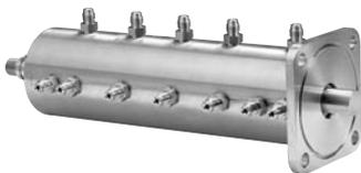
Ferrofluidic® rotary gas unions offer manufacturers of CVD and other deposition systems an efficient and flexible method of introducing gases into a process. A static gas feed runs into the rotating shaft which supports the wafer. This ensures that the gas outlet is in the center of the wafer, resulting in uniform coating characteristics.
