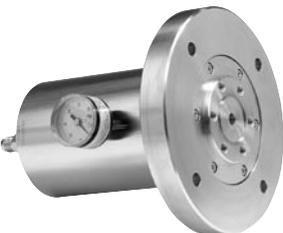
Reactive gas seals for applications such as MOCVD use an inert fluorocarbon based fluid. They feature a cantilevered seal design to protect the bearings from process gases. Special materials are used in the seal construction. Inert gas purges or protective plating can also be added to prevent corrosive attack of seal components.
